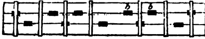
Fig. 61—Represents a solid built beam with keys b, b of hard wood between the courses.
